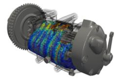
nanoFluidX is a particle-based fluid dynamics simulation tool to predict complex flows in complex geometries, such as the oiling in powertrain systems with rotating gears.
