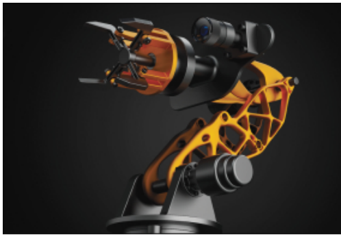
Robot arm designed and optimized using Inspire
