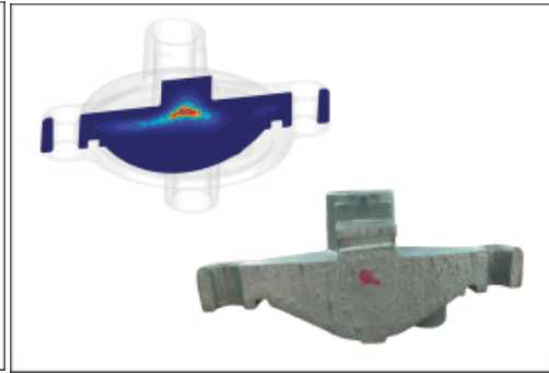
Fast and accurate casting defect prediction
