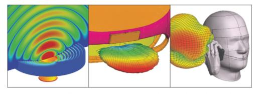
EM simulation of corrugated horn antenna to ensure total system performance
