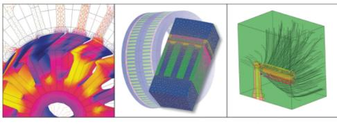
Flux density simulation of an induction machine to optimize electric motor performance
