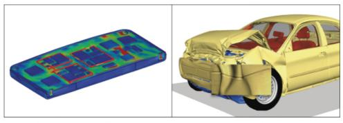
Printed circuit board deformation during smart phone drop test
