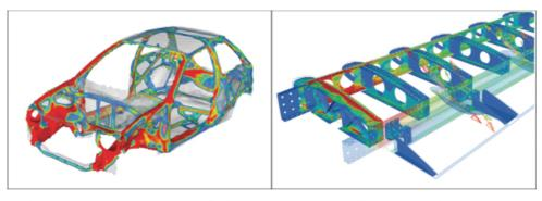
Car frame designed with topology optimization to maximize performance and minimize weight
