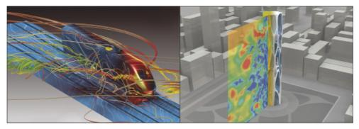
Rail car pressure field and streamlines from drag-reduction simulation
