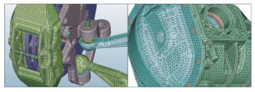
Full system vehicle suspension finite element mesh
