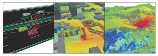
Radio network propagation analysis for interconnected vehicles
